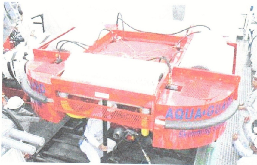
Fig 3.1 – Typical Oil Skimmer
